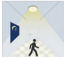
WHEN AMBIENT LIGHT IS DIM, SENSORS DETECT MOTION AND LIGHTS ARE 100% ON.
