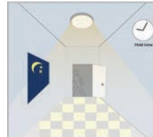
WHEN THE HOLDING TIME ENDS AND NO MOTION IS DETECTED, THE LIGHT BRIGHTNESS IS AUTOMATICALLY DIMMED AND THE WAITING TIME STARTS.
